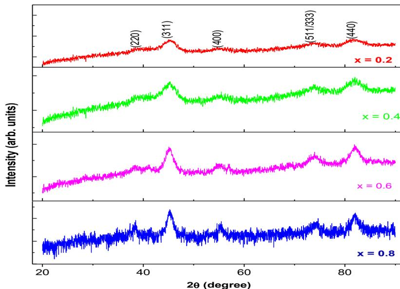
**Figure1. The XRD Pattern Obtained For The Samples**
