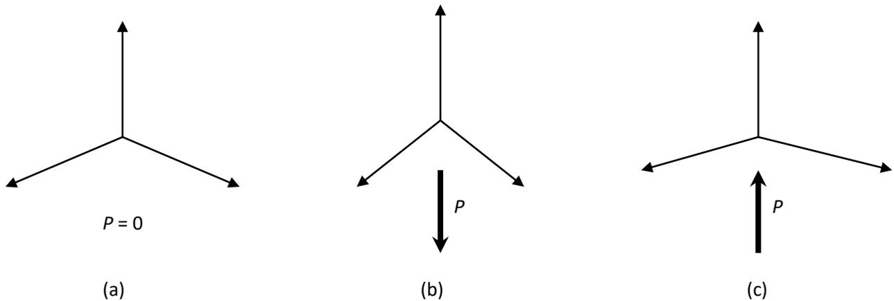
Fig. 1 (a) Directions of polarization (b) A vertical tension or a horizontal compression causing (c) A vertical compression or a horizontal tension causing a net polarization
