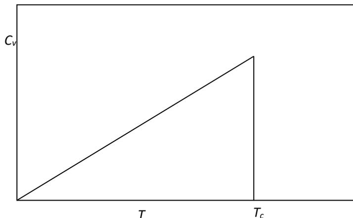
Fig. 2 Temperature dependence of specific heat showing anomaly at a second-order phase transition
