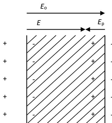
**Fig.1.** Effect of polarization in a dielectric.
