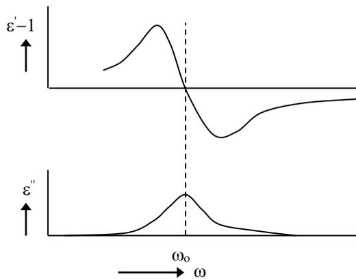
Fig.3 Behaviour of  $\epsilon'_o$  and  $\epsilon''_o$  as function of frequency in the vicinity of the resonance frequency  $\omega_0$
