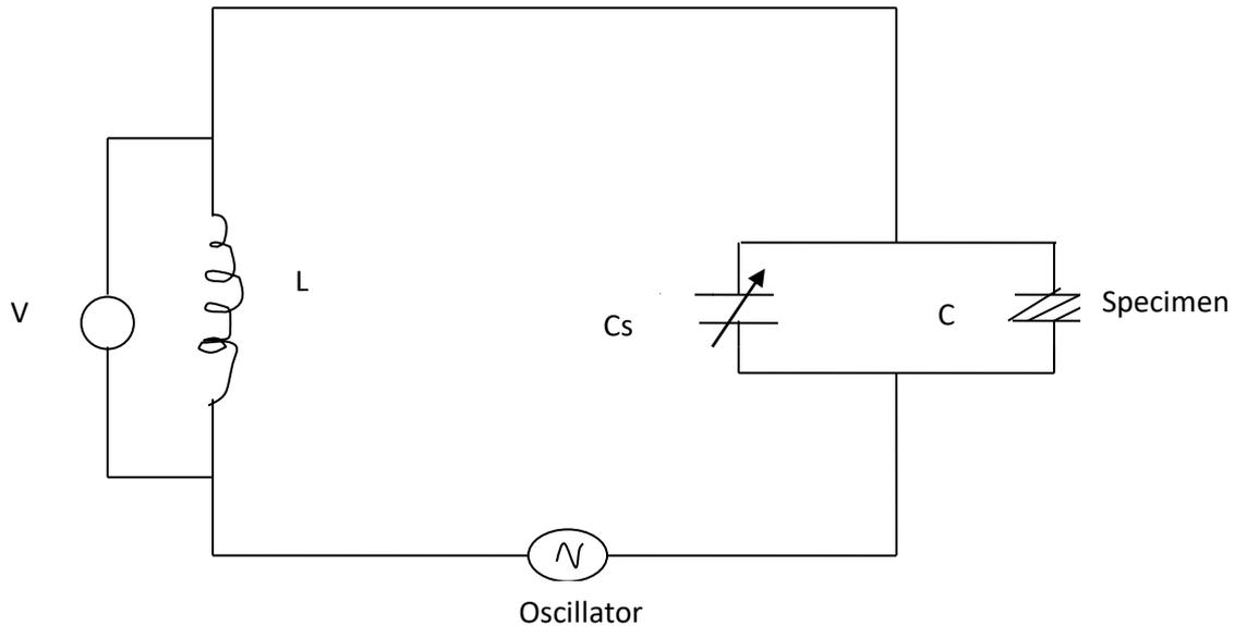
**Fig. 5** Principle of the resonance method for measuring  $C_0$  and  $C_d$ .
