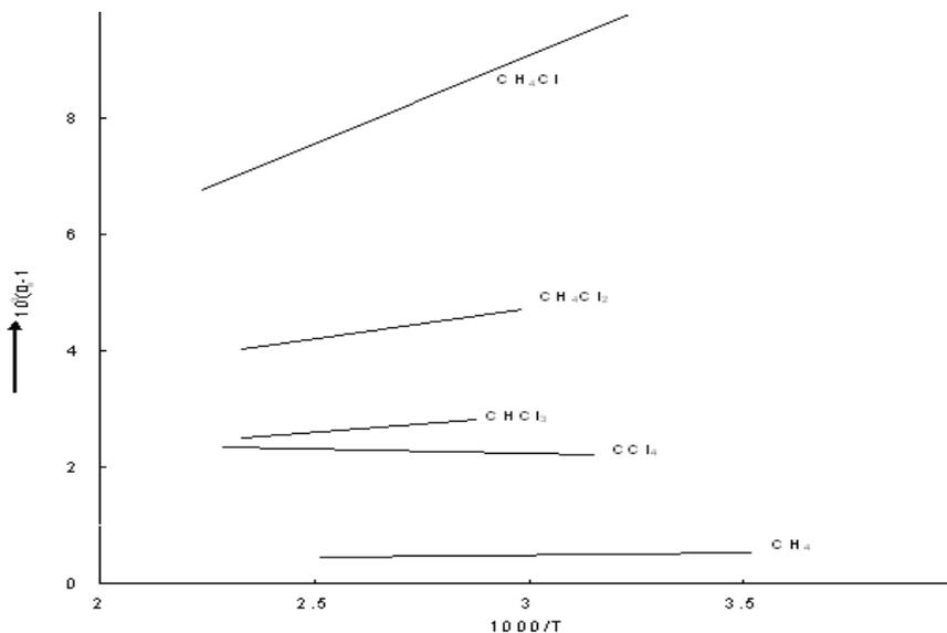
**Fig.1** Temperature variation of the static dielectric constant of some vapours.
