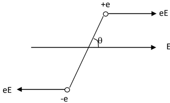
**Fig. 5** Torque applied by a field on a dipole.
