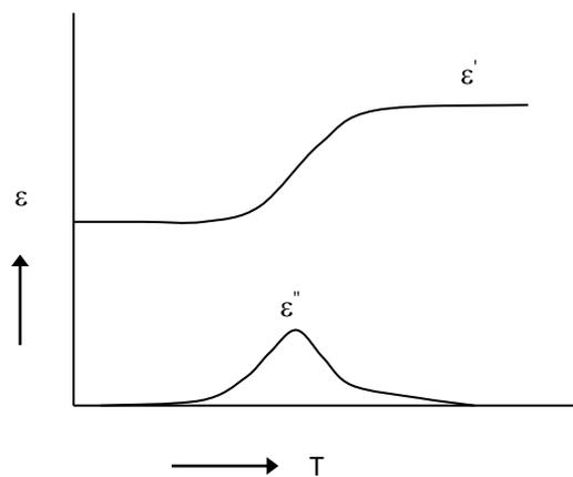
**Fig.2** The dielectric constant as a function of temperature at a given frequency, as predicted from the model discussed in the text
