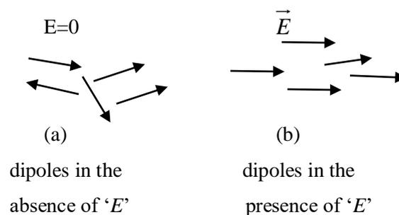
**Fig. 4.** Orientational polarization.
