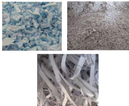
Fig 2. Bulk waste specimen used clockwise from top left, Polysterene, Sawdust and Hredded waste paper (Source: Vasilache, Maricica & Pruteanu, Marian & Avram, Costel, 2010 pg.1277
